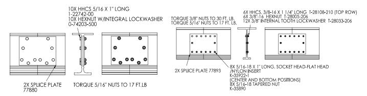
Diagram 4H. Bolted splice (4200 - 4600 Tarca® beam).
