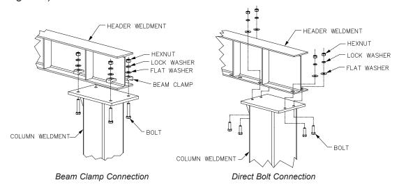
Diagram 3B. Installing header weldments.
