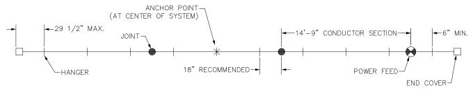
Diagram 12D. Typical conductor bar.
