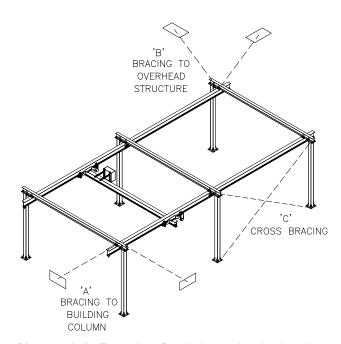
Diagram 14A. Examples of typical sway bracing locations.
