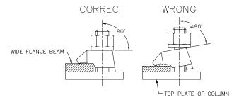
Diagram 3C. Beam Clamp Installation.
