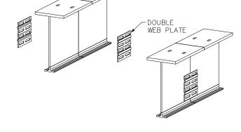
Diagram 4E. Welded splice (4200-4600 Tarca® beam).
