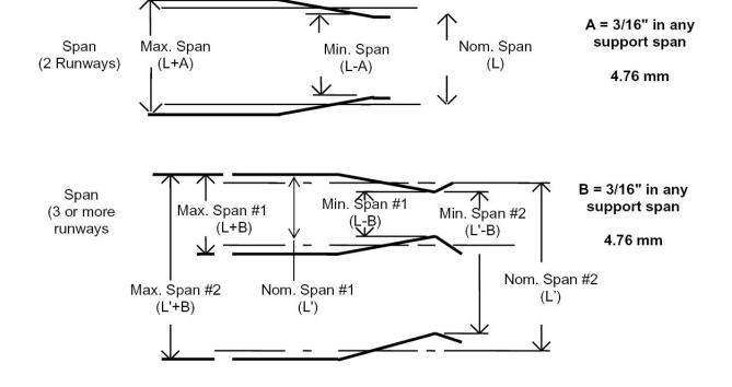
Diagram 4K. Runway alignment tolerance.
