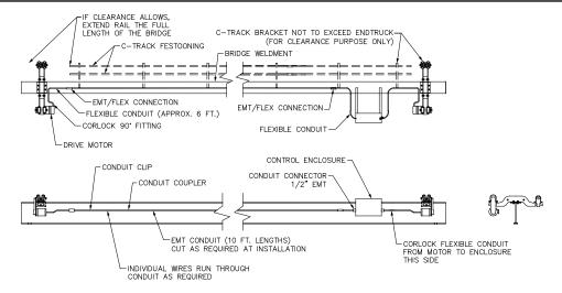
Diagram 10A. Bridge conduit wiring diagram.
