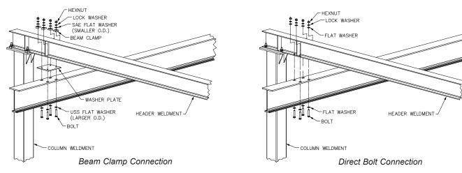
Diagram 4A. Attaching runway to header weldment.
