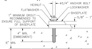
Diagram 1A. Typical anchor bolt embedment.
