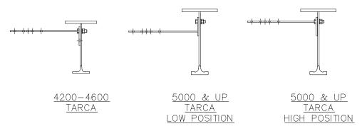
Diagram 12A. Conductor bar mounting bracket.
