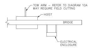
Diagram 7E. Standard tow arm orientation (top view).
