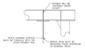
Diagram 4B. Track Perpendicularity.
