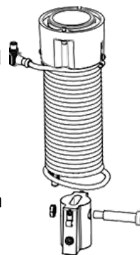
Diagram 2-4A. Standard Coil Cord Assembly
