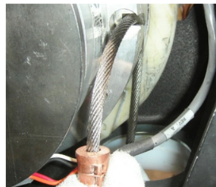
Diagram 7-8. Insert rope from actuator through opening at bottom & form loop to set in radius channel.
