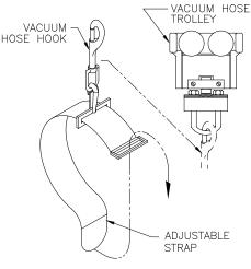
Diagram 4B. Installing vacuum hose on vacuum hose trolley.
