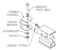
Diagram 2E. Attaching lower pivot assembly to lower formed channel.
