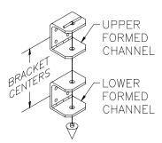
**Diagram 2A.** *Plumbing* formed channel brackets.
