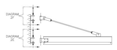
Diagram 2G. Attaching aluminum jib to formed channels.
