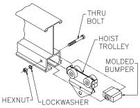
Diagram 3H. Installing hoist trolley and endstop.
