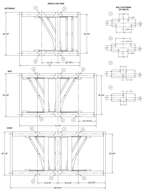
Diagram 2A. Switch support detail.
