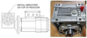
Diagram 6A. Installing breather on top of reducer.
