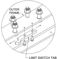
Diagram 6D. Limit switch tab for plunger limit switch (on 3 Way Switch only)
